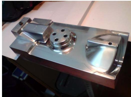
The hull and deck have laminated with two layers fabric of 165 grams/m<sup>2</sup> twill Sglas, joined both semihulls for two tapes of reinforcement of 20m/m of 200 grams/m<sup>2</sup>. The used resin is epoxy Ampreg 26, of SP systems. Previously in the surface of the mold the gelcoat has been applied by spray (to unify the thickness and to save weight), reflecting the polished brilliant one of the mold in the finished superficial one.
